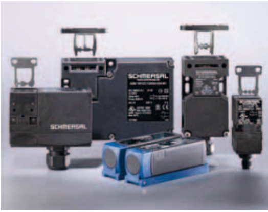
Fig. 3 In the case of safety switches – also referred to as class 2 switches – the switching element and actuator are not connected structurally to each other but are functionally joined or separated during switching. The actuator is separated from the basic unit when the protective device is open. Here, NC contacts in the safety switch are positively opened and NO contacts are closed.
