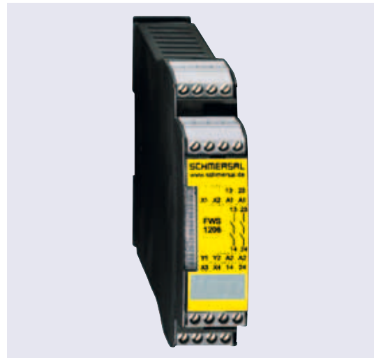
Fig. 3 The shut-down monitors from the FWS range serve to safely record the machine’s shut-down. Depending on the external circuit in conjunction with a safety monitoring module from the AES or SRB range, it is possible to safeguard a protective device up to PL “d”.
