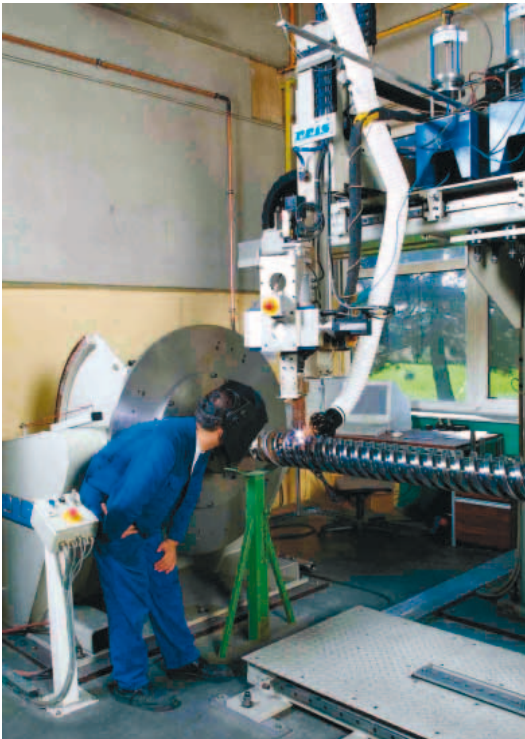
Fig. 7 Observation of processes, e.g. for overlay welding during reprocessing of the extruder screws.
