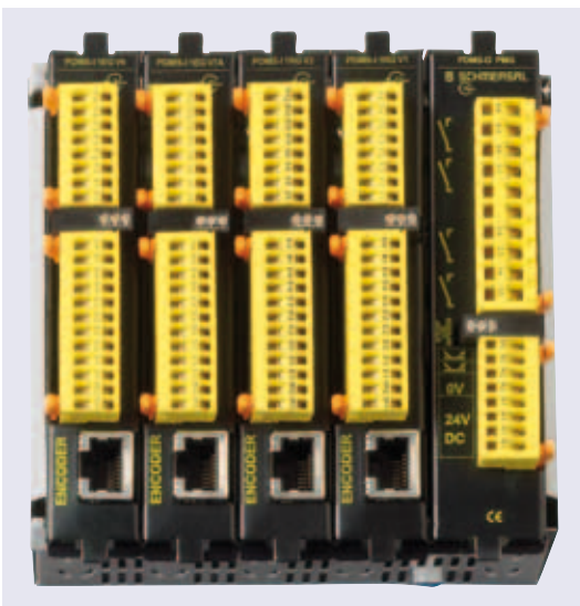
Fig. 9 The “Protect Drive Monitoring System” PDMS, a solution with modular structure for safe shut-down and speed monitoring, e.g. of spindle or final drives up to PL “e”, serves as an extension to the universally applicable PROTECT PSC safety controller.
