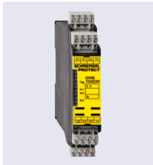
Fig. 9 Safety module SRB 100DR with double acknowledgement, for example, ensures additional safety in accessible hazardous areas. The module ensures that the machine control system can only be switched back on once the operator has left the hazardous area. This is because the operator must firstly actuate a reset or restart button located inside the system, followed by a second which is positioned outside the accessible hazardous area.
